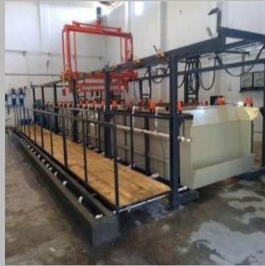
Hard Chrome Electroplating Plant
