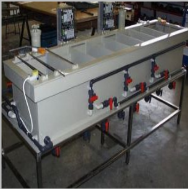
Nickel Electroplating Plant
