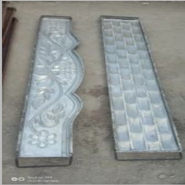
Boundary Wall Mould
