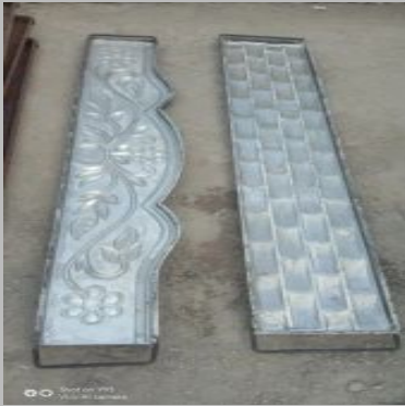
Boundary Wall Mould
