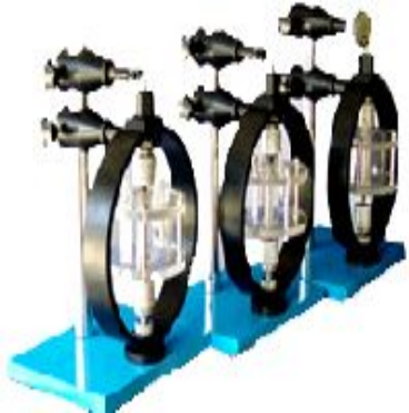
Stress Corrosion Cracking SSCC proof rings as per NACE TM0177-96
