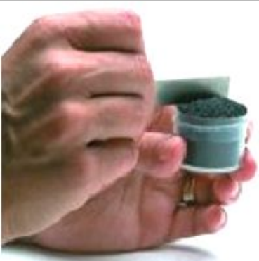
Chloride Ion Test
