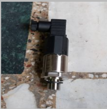
Huba Pressure Transmitter Model 528.8140032411W RANGE 0-2 BAR
