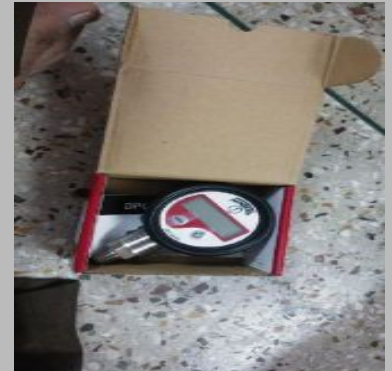
Winters Digital Pressure Gauge Model No DPG222R11
