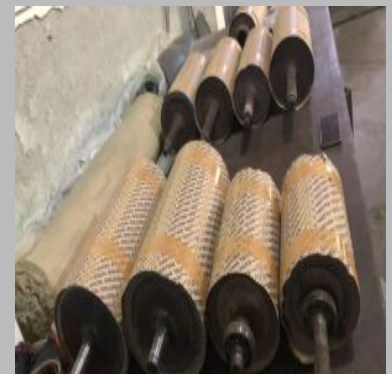
Mild Steel Leather Processing Roller
