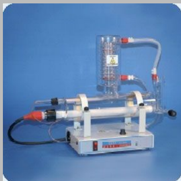
Water Distillation Unit with silica Heater 2 Ltrs/Hr
