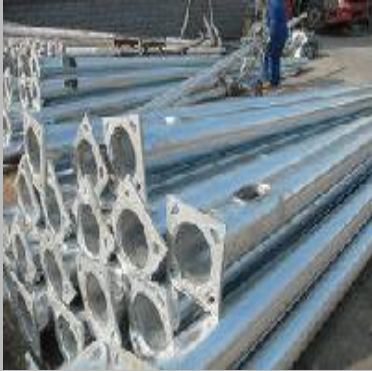
polygonal poles Galvanized
