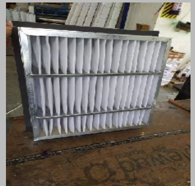
AHU Air Filter
