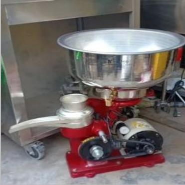
Stainless Steel Hand Cum Electric Milk Cream Separator
