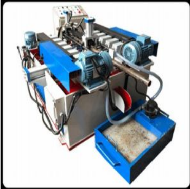
Scaffolding Drilling Machine
