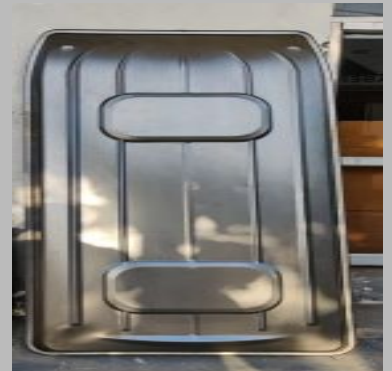
E- Rickshaw Roof Frame
