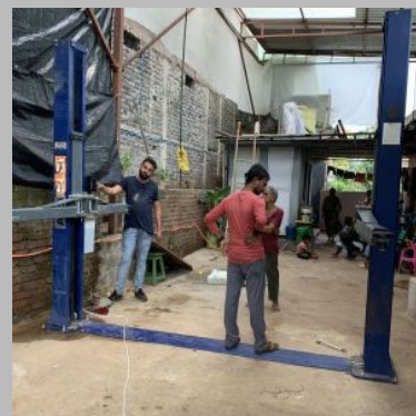
Mild Steel 4 Ton Clear Floor Hydraulic Two Post Lift
