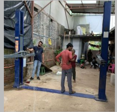
Mild Steel 4 Ton Clear Floor Hydraulic Two Post Lift
