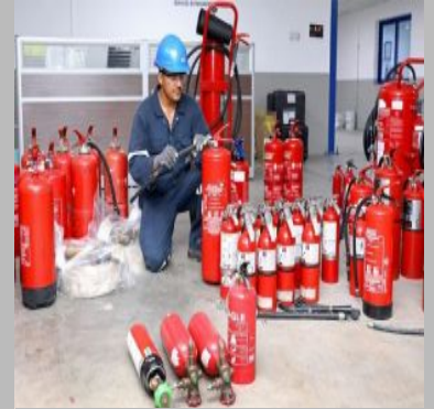
Fire Extinguisher Refilling
