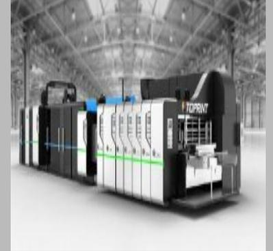
Flexo Printer Slotter Die Cutting With Inline Folder Gluer
