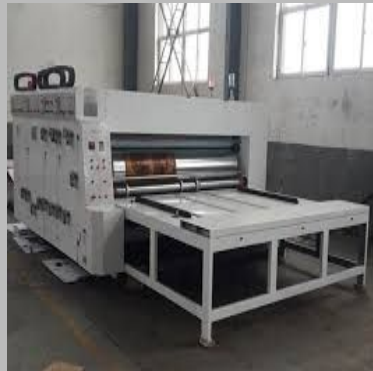
RNN-480 series two- color of water base printing slotting die- cutting machine
