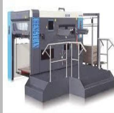
Semi-Automatic Flat Bed Die-Cutting Machine
