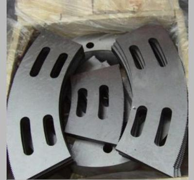
Slotting and Cutoff Blades and Knives For Corrugated Board Plant
