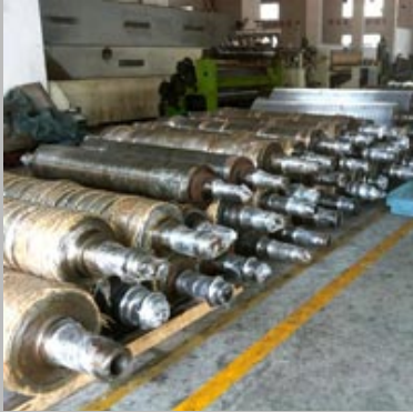
Corrugating Rollers Regrinding
