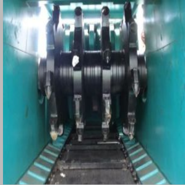
Surface Feeder Breaker
