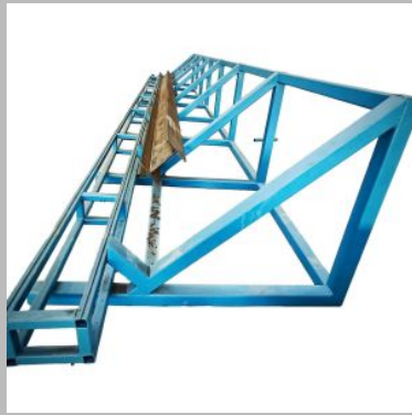
Saw Welding Stand with Mounted Track
