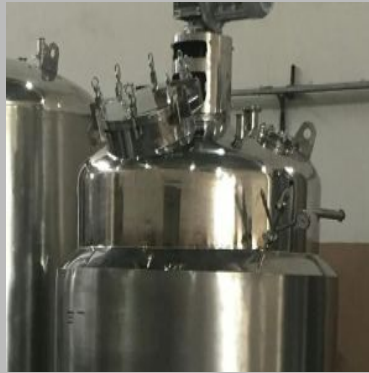
Jacketed Reactor Vessel
