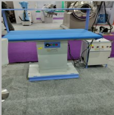
Vacuum Ironing Tables and Boiler
