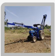
New Holland Tractor Fitted Pole Erection and Post Hole Digger
