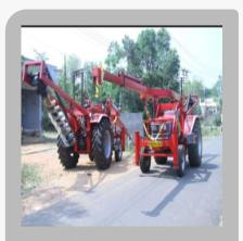
Mahindra Tractor Fitted Pole Erection Machine
