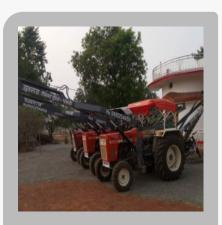
Swaraj Tractor fitted Pole Erection And Post Hole Digger
