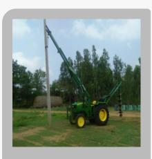
John Deere fitted Pole Erection Machine
