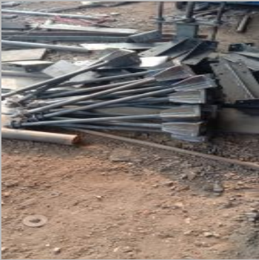
Plate type foundation bolt with stiffner
